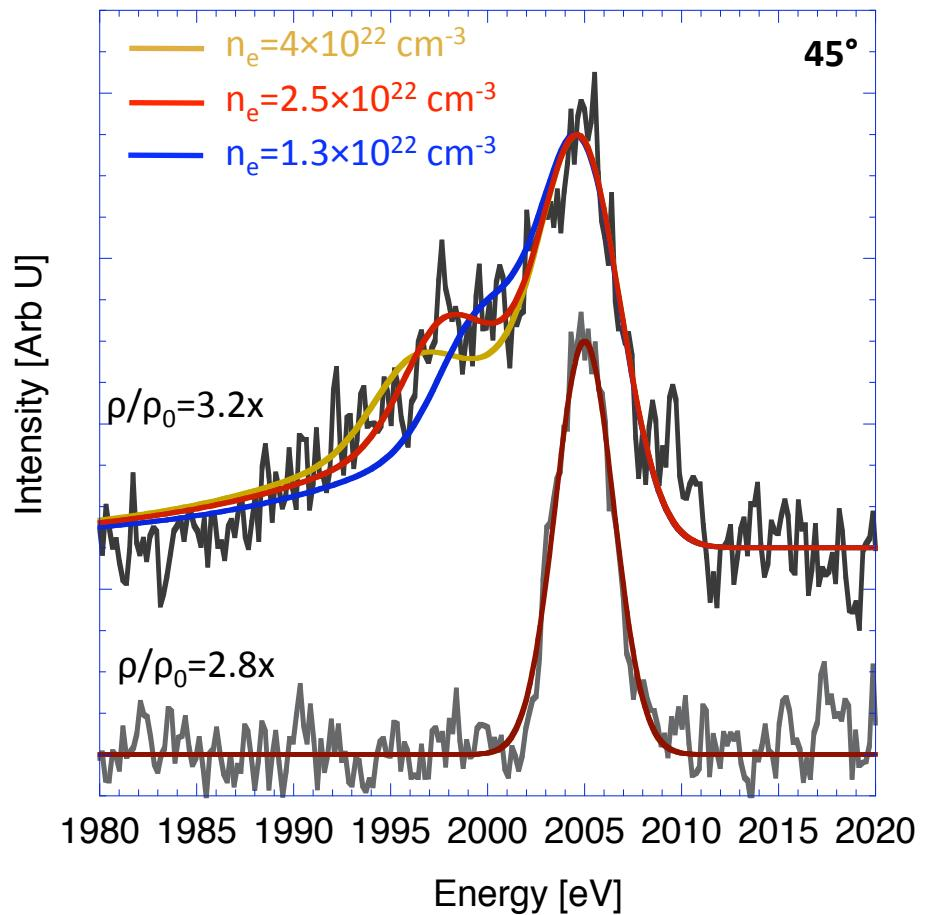
Backscattering spectrum corroborates onset of ionization
