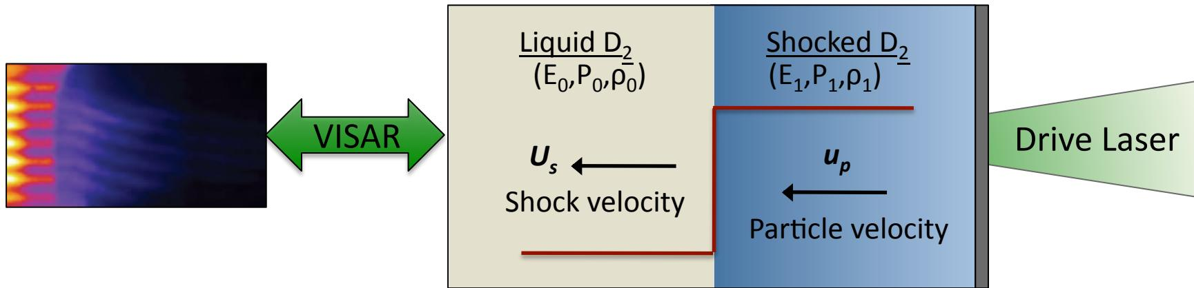
Since hydrogen is reflective at high pressure, velocity interferometry (VISAR) can be used to measure the shock velocity and infer material properties.
