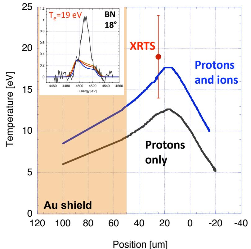
Detailed balance temperature measurement is consistent with hydrodynamic simulations
