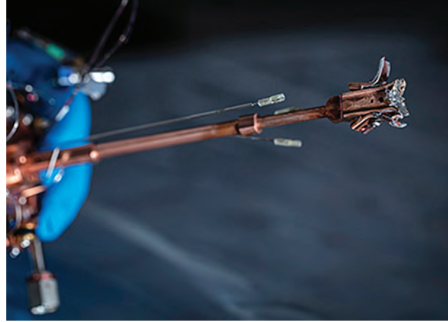
A NIF target (left) before an experimental shot and (right) after the facility's milestone ignition shot. The cylinder is a centimeter-wide hohlraum that contains a fuel capsule just millimeters in diameter. Lawrence Livermore National Laboratory.
