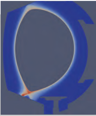
A snapshot of electron density for a simulated cross-section of a tokamak. Logan Meredith.
